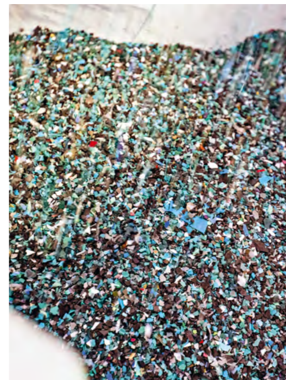
Raw Material: Discarded plastic products are being collected, shredded and washed for use in the production of Circleg prostheses.
